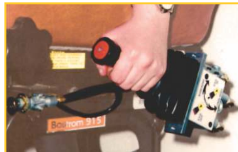
Operating the P.T.O. and Dump.
